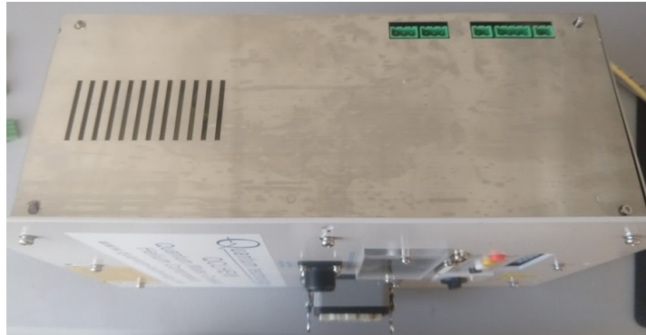
Figure 3: Side panel. Remove 4 screws to reach fuses
