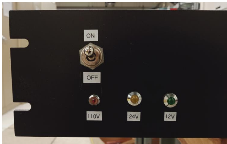
Figure 2: Front panel of the lifter control box
