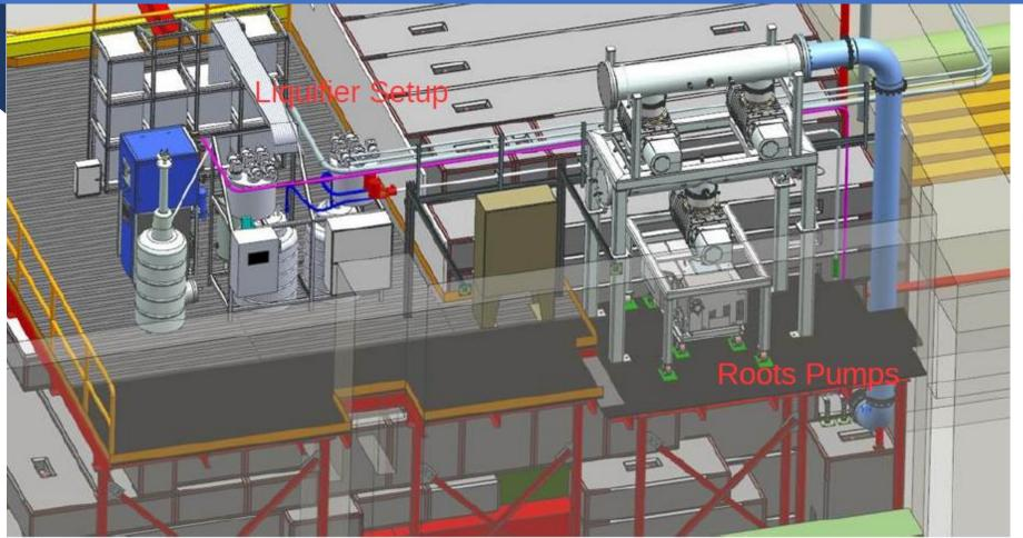
Cryo platform showing the He-liquefier and Roots pumps setup
