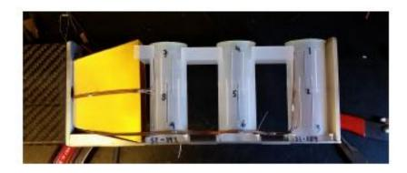
We will have 3 target cups so we can quickly replace the target when it is damaged due to the radiation
