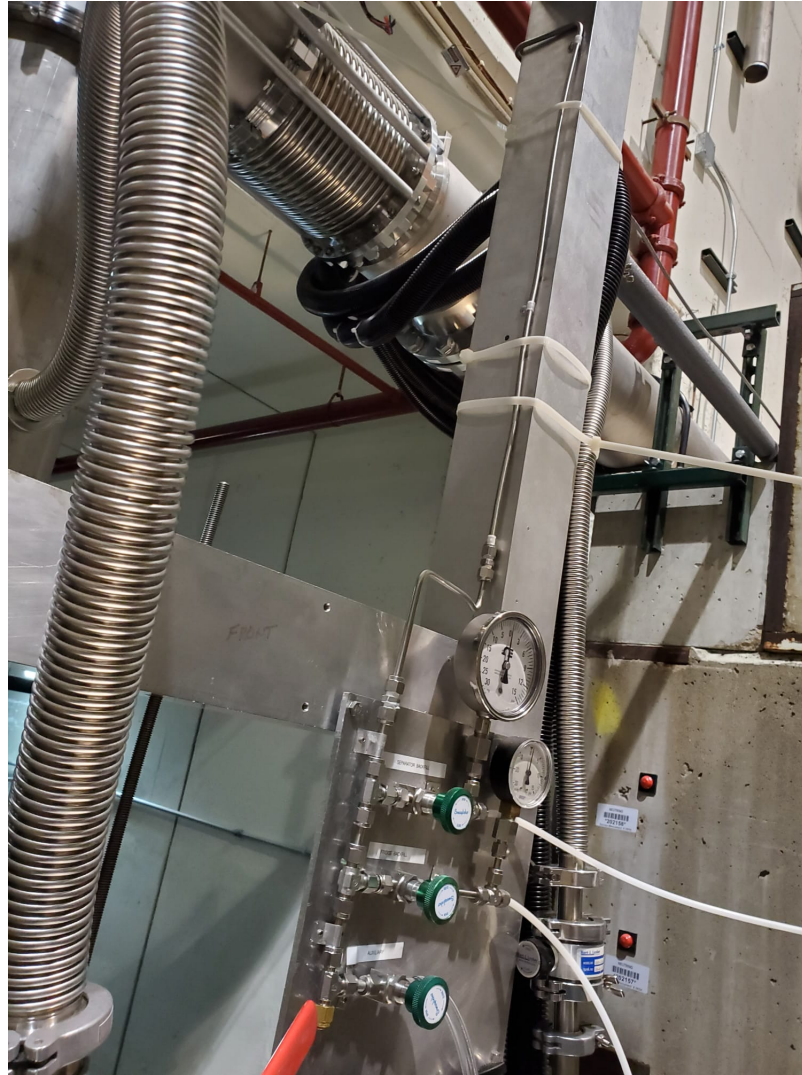
Helium backfill line connected to the panel: by Waqar & Ernesto
