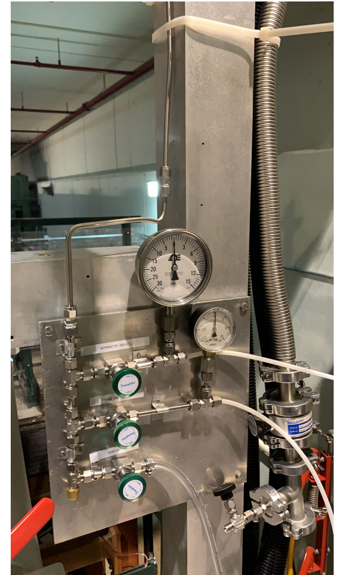
Helium backfill line connected to the panel: by Waqar & Ernesto
