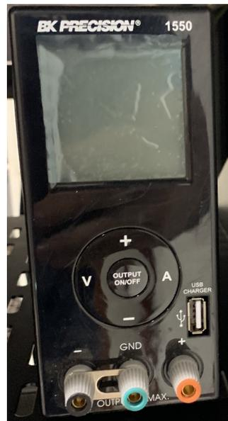
Figure 9: BK Precision 1550 power supply
