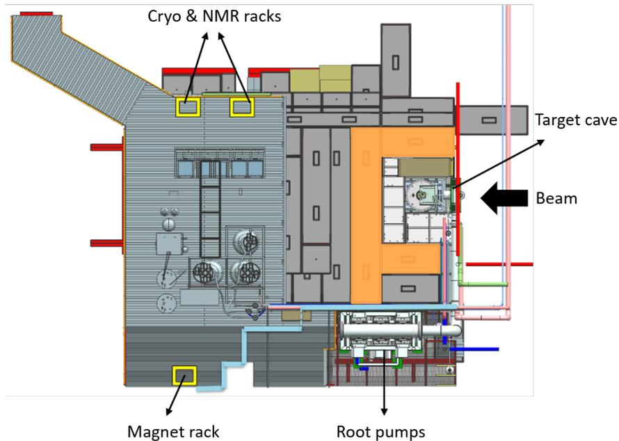
Figure 1: Top view of the cryo platform showing the location of the magnet rack, NMR rack, cryo or target (slow control) rack, root pumps and target cave.
