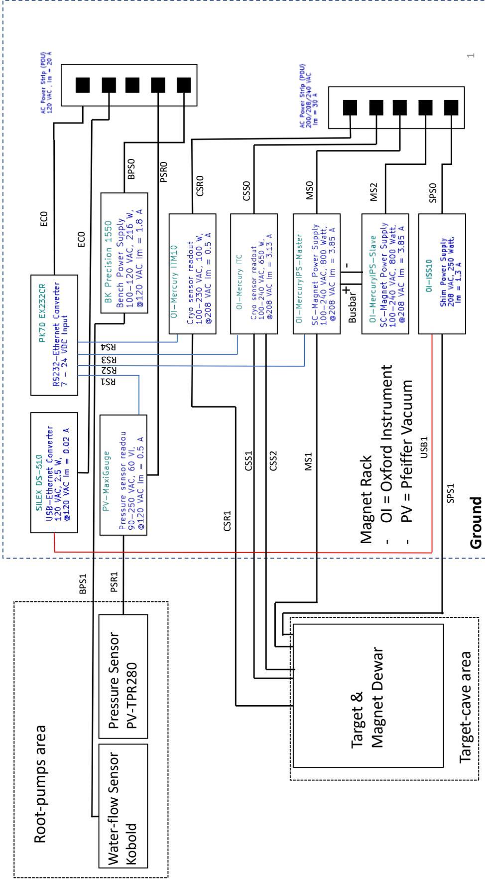
Figure 3: The layout and instruments housed in the magnet rack.
