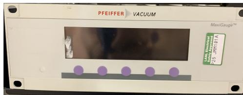
Figure 8: Multi channels Maxigauge pressure sensor read out from Pfeiffer Vacuum.
