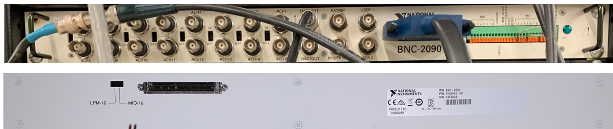
Figure 2.1.1: BNC 2090 (upper: front panel, lower: back panel)
