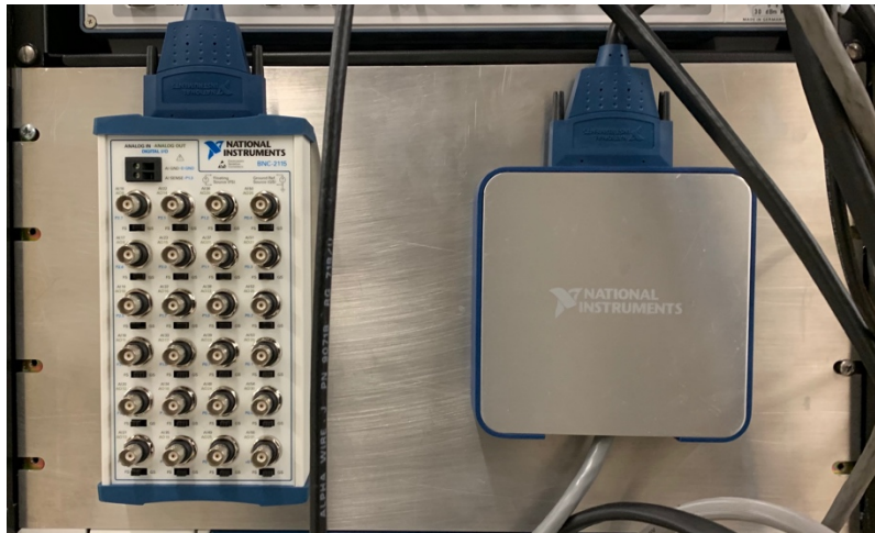
Figure 2.2.1: (left) BNC 2115, (right) SCB-668A
