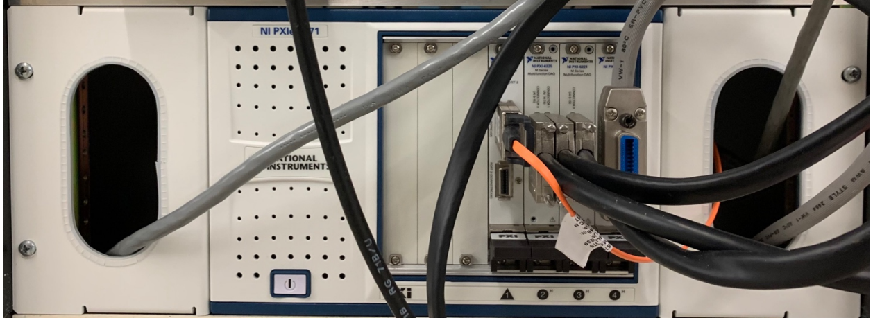
Figure 2.4.1: The PXI system (or the DAQ panel) of the UVA-NMR system
