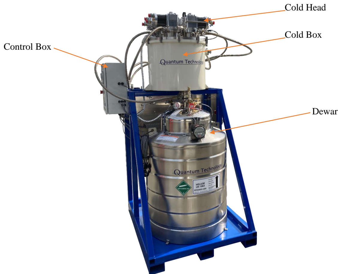
Figure 1: Liquefier Major Components
