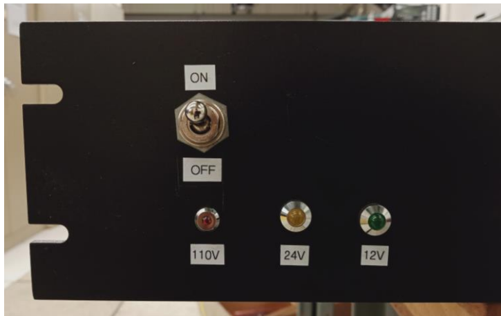
Figure 1: Front panel of the lifter control box
