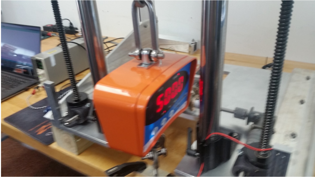
Figure 3 - Test setup showing the crane scale readout with 500 lbf load
