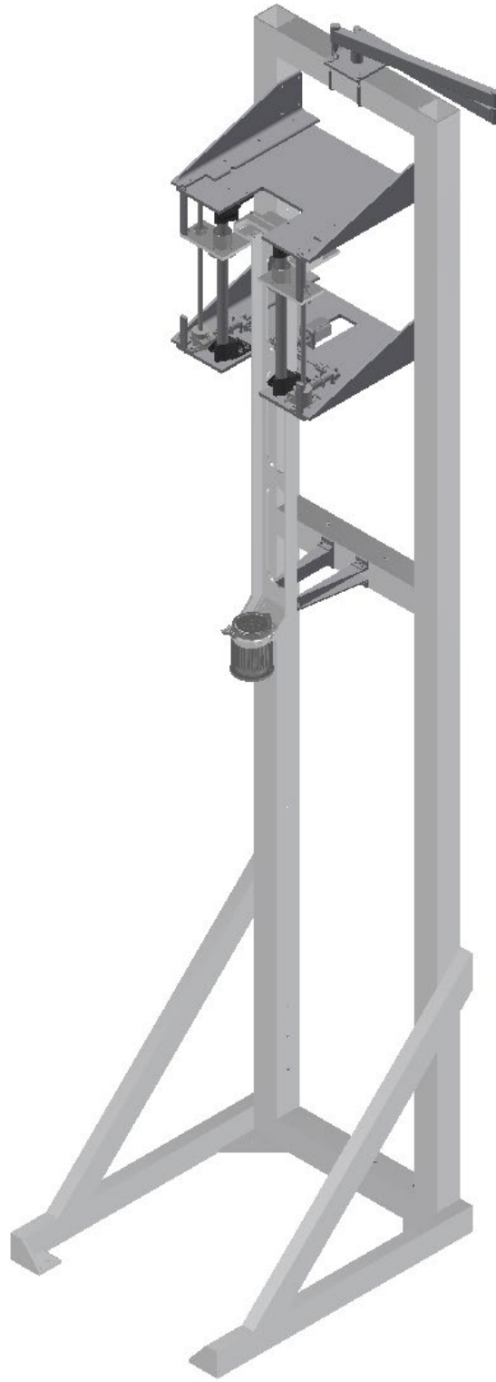
Figure 1- Overall design of E1039 target support frame and insert elevator assembly
