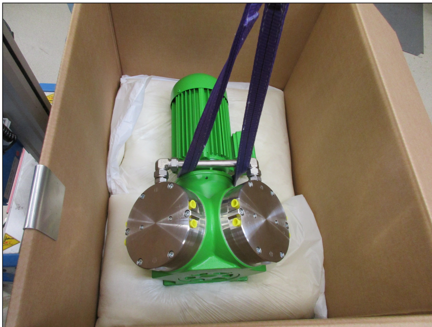
Fig. 6 Position of carrying strap (example)
