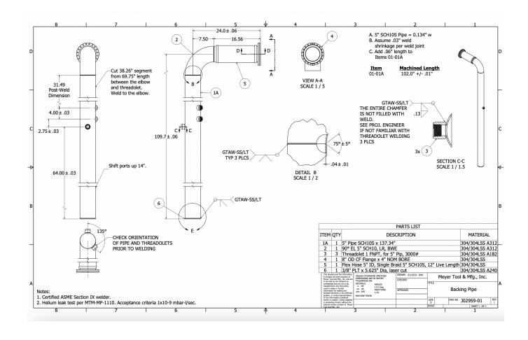
The Conflat flange and pipe welds were welded by FNAL welder Austin Fletcher. These welds took place as per the method given in ED0004253 and qualify built as per ASME B31.3.
